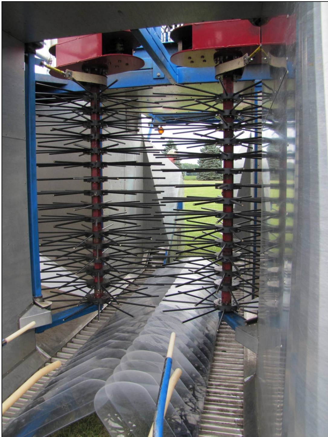
Interior view of a conventional blueberry harvester. The vertical spindles rotate to allow bushes to pass through, and also vibrate by the action of offset counterweights (in red housings at top) to shake berries free. Scale-like catch plates at bottom are spring-loaded to “flow” around bases of blueberry bushes to minimize berry loss by droppage. Conveyor belts on either side of the catch plates carry berries to the rear of the harvester to be deposited into plastic lugs.
