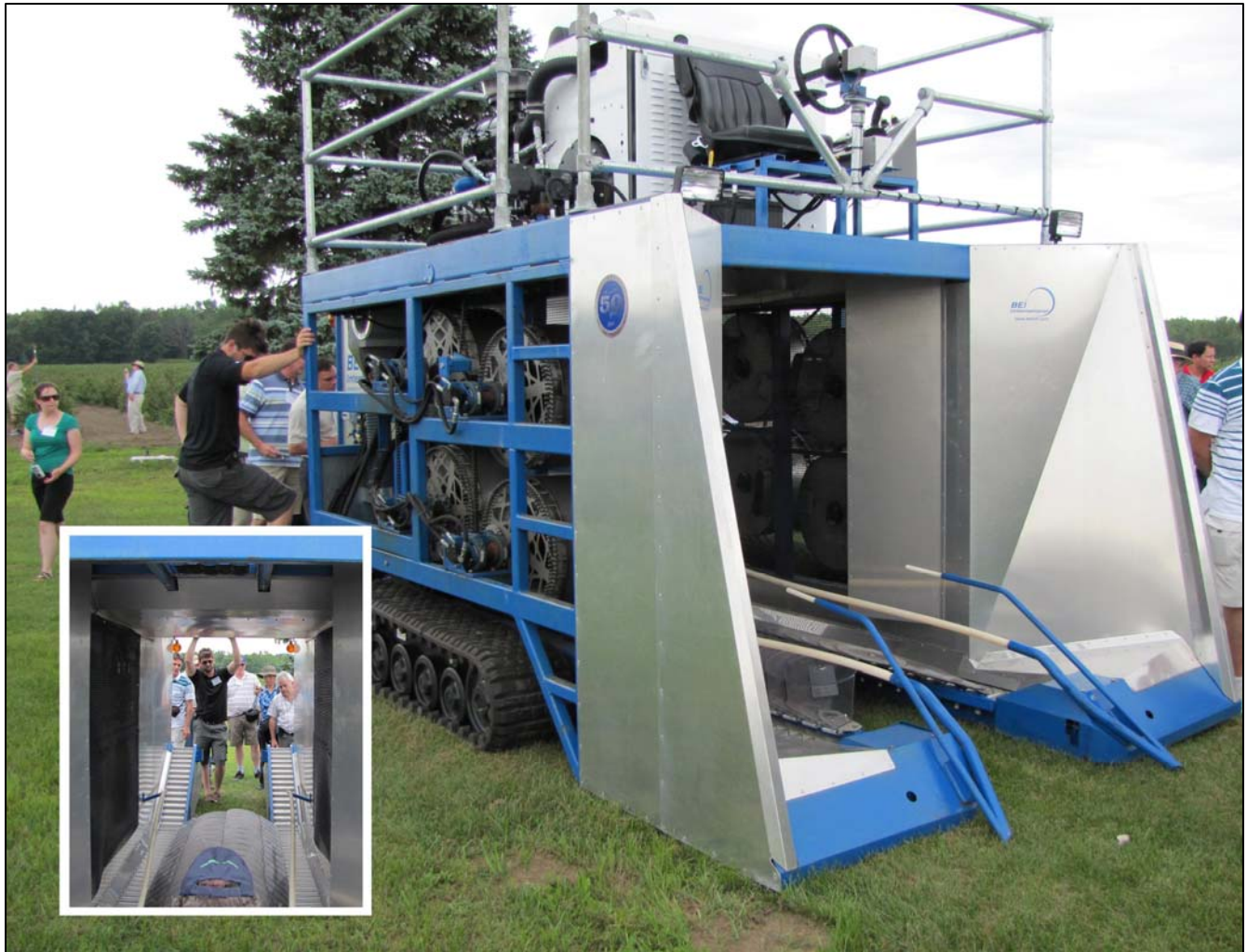
Exterior and interior view of a Black Ice™ blueberry harvester manufactured by BEI International, LLC (photographed 2010). Berries are separated from bushes by the action of four rotating fans mounted in each sidewall of the harvester. Catch plates and conveyor belts on bottom are similar to those in a conventional harvester.
